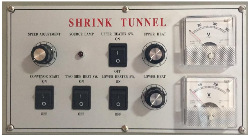
Figure 1. Control Panel of CN-4520A
